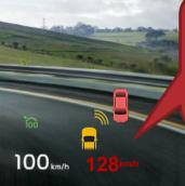
Remove irritating doppler audio and integrate radar into HUD
